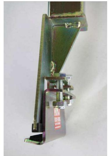
Next you can slide a cross bar through one side and add the bracket on the opposite side in turn. This method will help you ensure that the bars are running straight across your roof and also, it isn't possible to fit the rear door guard and front wind deflector bars any other way. (Make sure the deflector bar is facing the right way, as there's nothing worse than not deflecting your wind properly.)
